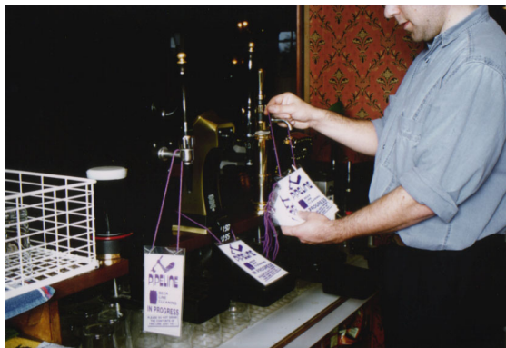
CIP Cleaning in Progress
